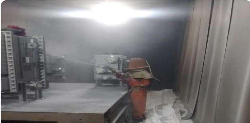
Multiple Shotblasting and Painting Booths
