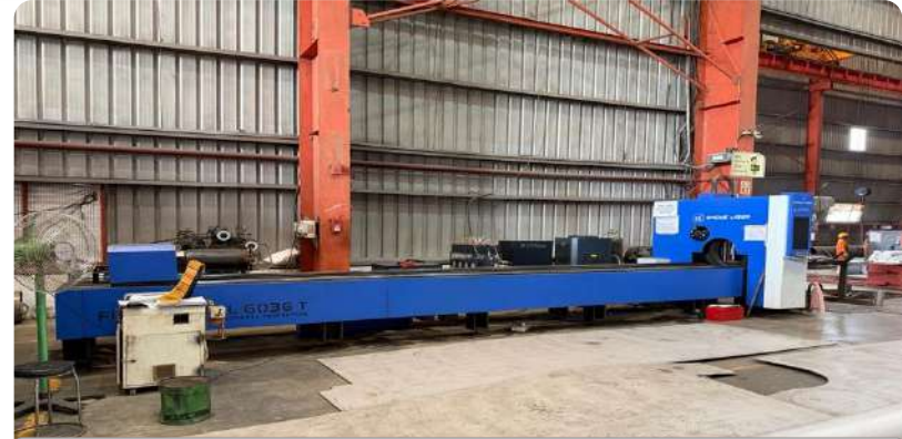
Laser Pipe Cutting Machine: Up to 14" OD
