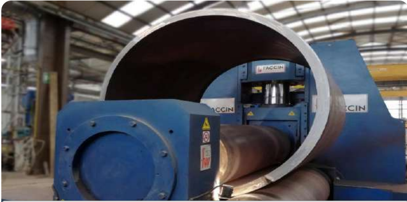
Rolling Machines: 3 Roll, CNC Controlled, 100 mm x 3000 mm
